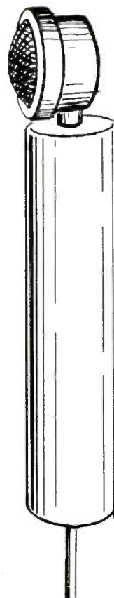
Figure 2. The condensor microphone followed the carbon type and provided many advantages in fidelity.
